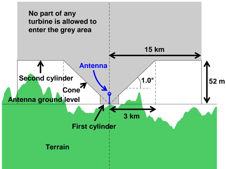
Figure 3-5: Illustration of the CVOR safeguarding zone in side view. The drawing is not to scale. Blue line = antenna. Green area = terrain. Grey area = zone where turbines are not allowed
