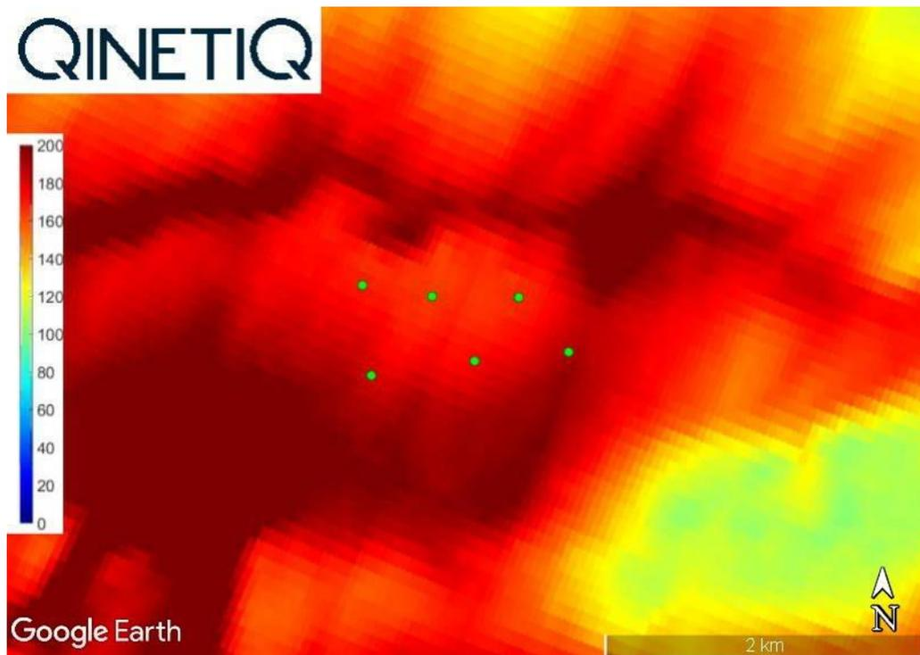
Figure 2-1: Height to LoS (m AGL) as viewed from the Beauvechain PSR. Green dots = proposed turbines
