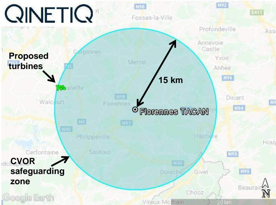
Figure 3-3: Safeguarding zone (blue) for the VOR sub-system, using the criteria for a CVOR. Green dots = proposed turbines
