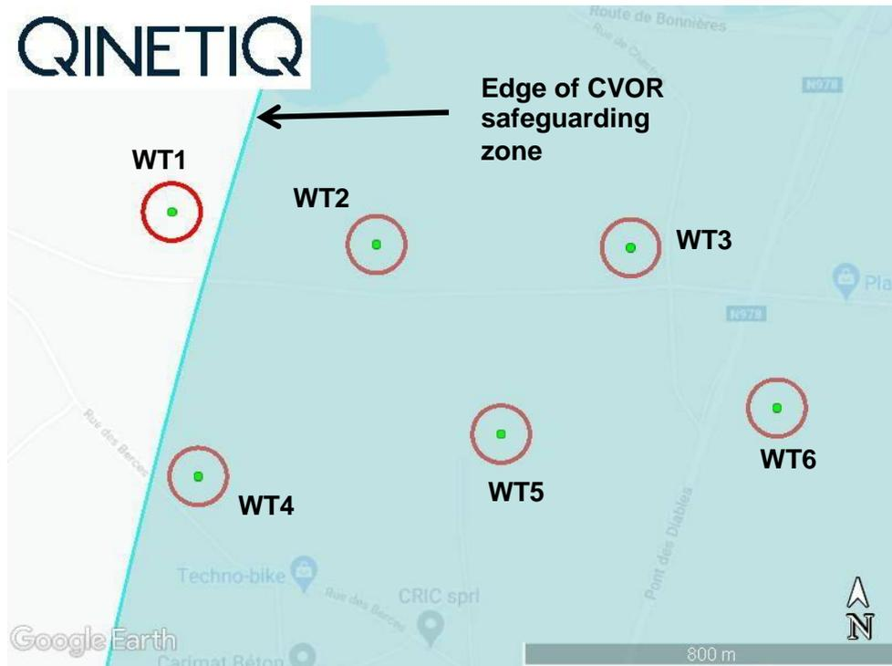
Figure 3-4: Close-up view of the CVOR safeguarding zone in the vicinity of the proposed turbines (green dots). Red circles = rotor sweep area, using a rotor diameter of 122 metres
