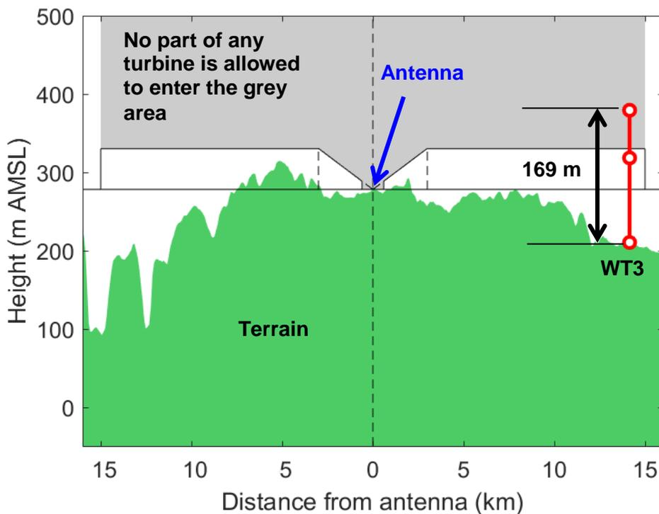
Figure 3-6: Turbine WT3 in relation to the CVOR safeguarding zone. Green area = terrain. Grey area = zone where turbines are not allowed. Red line = vertical extent of turbine, assuming 169 metre maximum height. Red circles indicate the ground elevation, hub height, and maximum blade tip height
