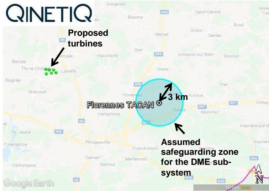
Figure 3-2: Safeguarding zone (blue) for the DME sub-system, assuming the criteria for an omni-directional DME. Green dots = proposed turbines
